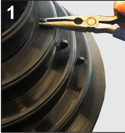
1 Break off knob with needle nose pliers at level of chosen size
